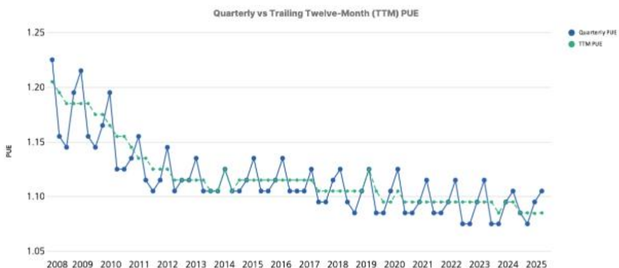
Abbildung 1: Power Usage effectiveness – Google Data Centers. Quelle: Google 2026.
