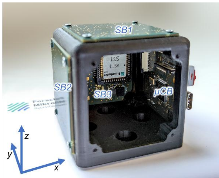
Fig. 3.2: ENAS-IMU with individual MEMS sensors (3x1-axis MEMS gyroscope, 3x2-axis MEMS accelerometer)
