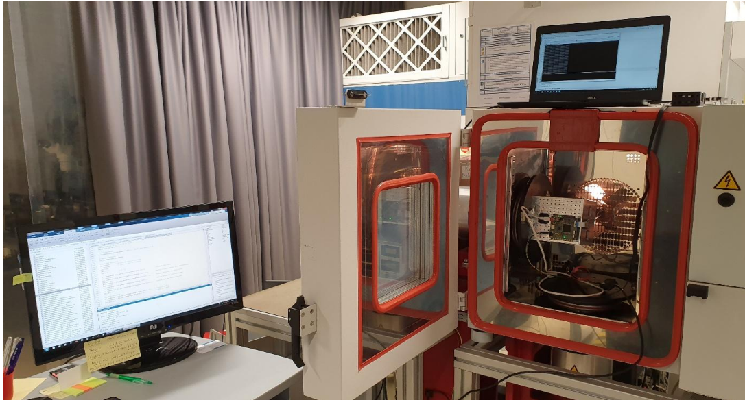
Fig. 3.1: Inertial measurement station consisting of AC1120S rotary table from Acutronic, temperature chamber from Vötsch and control computer
