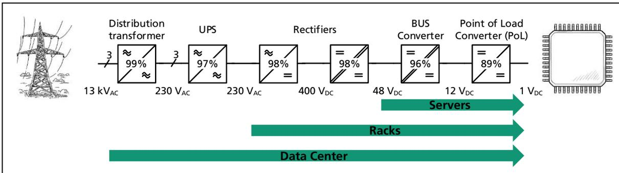
Figure 1: Block diagram of a power supply system for a data center.
