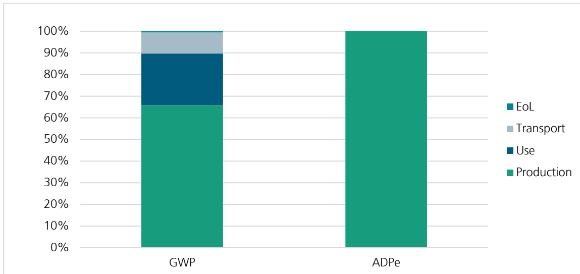
Figure 5-1: Relative impact of life cycle phase to the total impact per impact category
