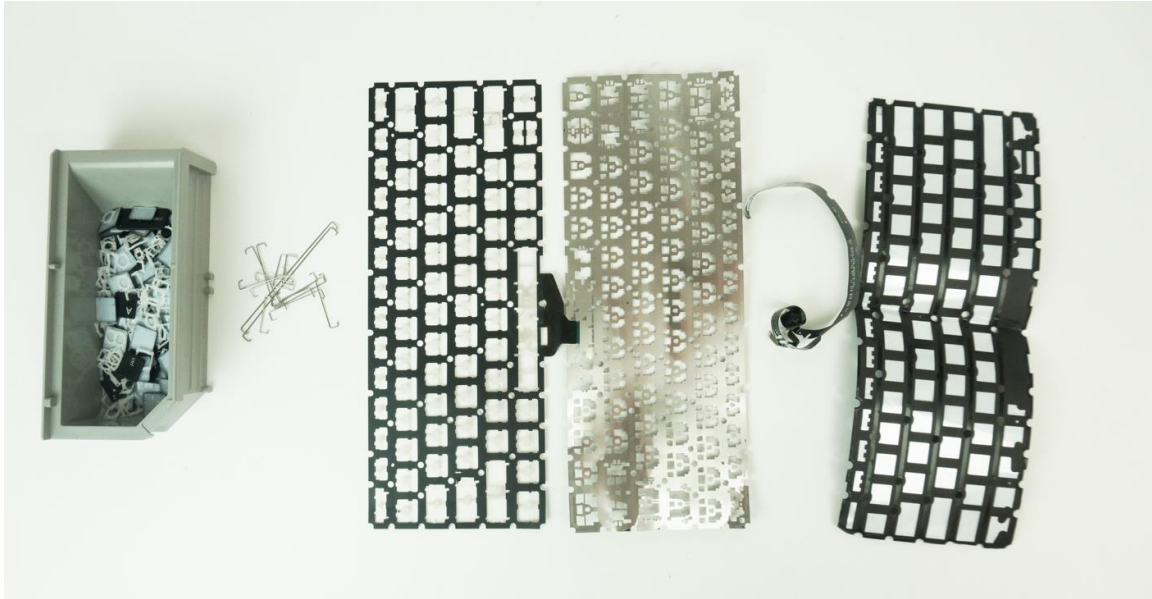
Figure 4-2: Teardown example of the keyboard module
